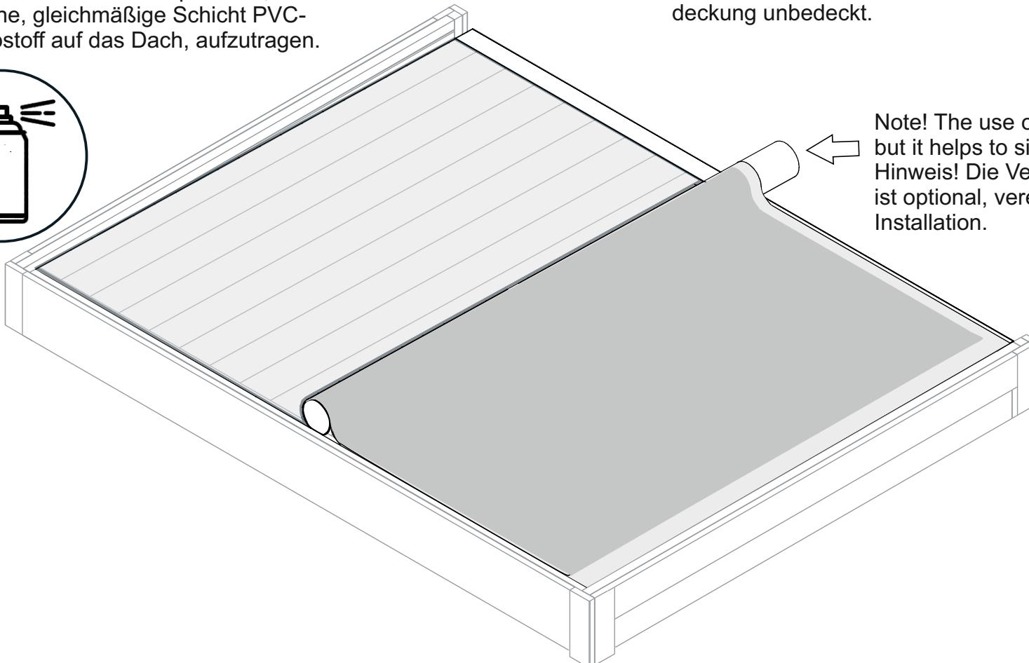
2. Apply adhesive to the PVC membrane, leaving the edges and the area near the rear flashing uncovered.
